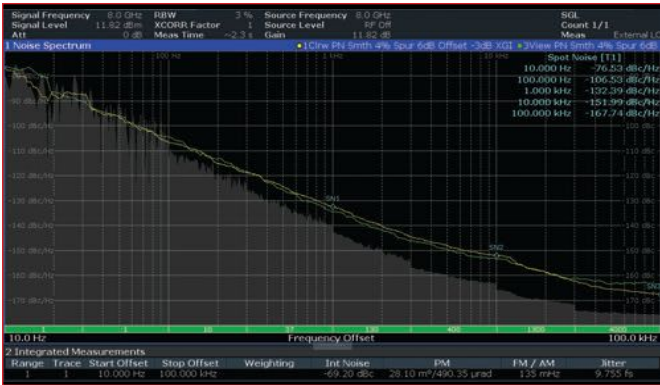
▲ Fig. 2 Typical measurement of two SLCOs, applying the two DUT method.
