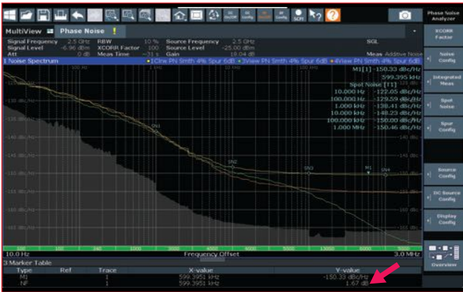
▲ Fig. 3 Additive/residual phase noise of an amplifier.
